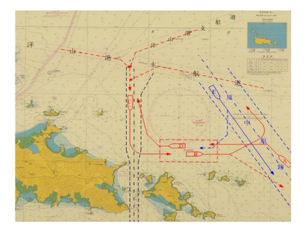
6. Diagram of the main bunker supply anchorage in Zhoushan
